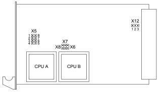
Jumpers X6, X7 and X8 must be not connected (no jumper placed).
