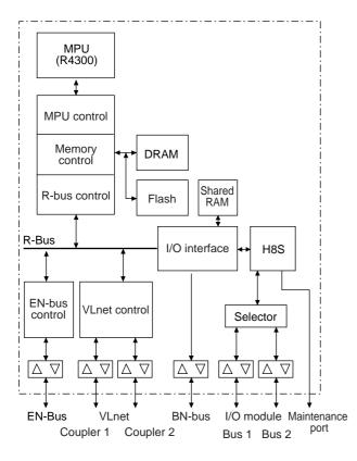
Figure 2 Internal Block Diagram of CPU Card
