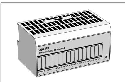
I/O unit for eight three-wire RTD input signals with programmable filters and 16-bit resolution. A number of sensors are supported. One bi-coloured LED indicates function status.
