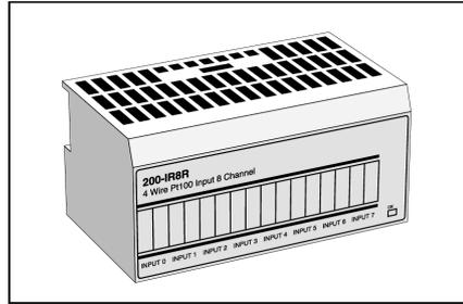
I/O unit for eight four-wire RTD input signals. The inputs have programmable filters and 16-bit resolution. One sensor type is supported.
