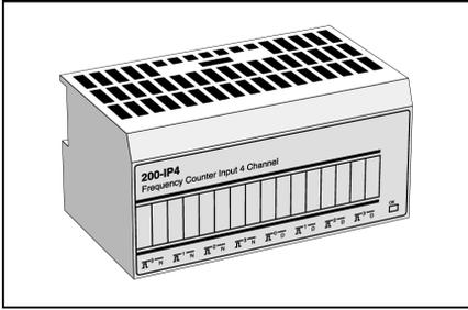
I/O unit with four pulse transmitter interfaces, each with two optocoupled inputs. The maximum pulse frequency is 100 kHz. The I/O unit is configured using the control system program.
